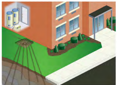
EarthLinked® Water Heating system with diagonal earth loop configuration.
