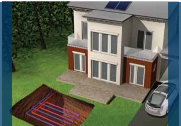
Horizontal Ground Loop System
